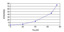
Therefore, the PF should move the tiller smoothly and maintain the tiller's position. Any correction should be small and smooth, and maintained for enough time to enable the pilot to assess the outcome. Being over-active on the tiller will cause uncomfortable oscillations.
