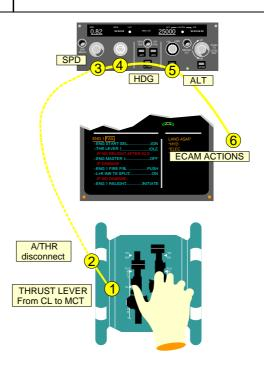
The A/THR is disconnected to avoid any engine thrust reduction when selecting speed according to strategy or when pulling for OPEN DES to initiate the descent. With the A/THR disconnected, the target speed is controlled by the elevator when in OPEN DES.
