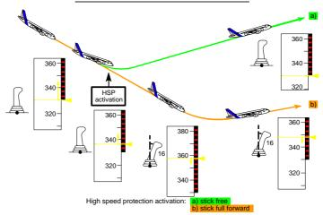
The PF, therefore, has full authority to perform a high speed/steep dive escape maneuver, when required, via a reflex action on the sidestick.
