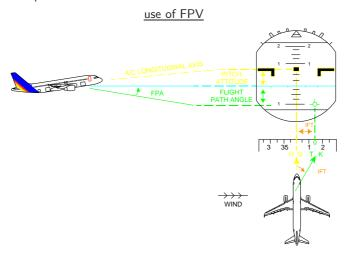
With the flight directors (FDs) selected ON, the Flight Path Director (FPD) replaces the HDG-VS Flight Director (FD). With both FDs pb set to off, the blue track index appears on the PFD horizon.
