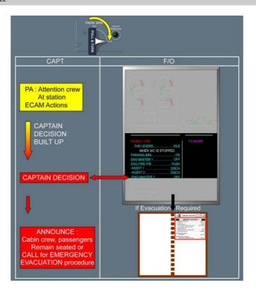
When applying the **EMERGENCY EVACUATION** procedure, the F/O can select the engine masters OFF and push the FIRE pb, without any confirmation from the Captain.
