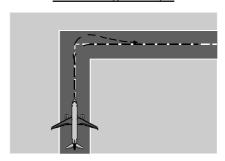
When exiting a tight turn, the pilot should anticipate the steer out. Additionally, the pilot should allow the aircraft to roll forward for a short distance to minimize the stress on the main gears.
