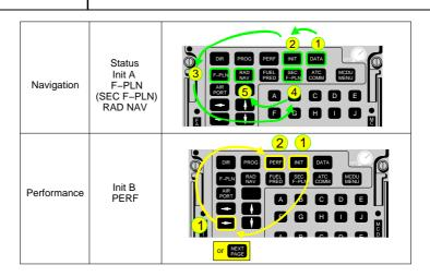
This sequence of entry is the most practical. INIT B should not be filled immediately after INIT A, because the FMGS would begin to compute F-PLN predictions. These computations would slow down the entry procedure.
