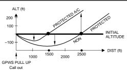
The above-illustrated are typical trajectories flown by all protected or not protected aircraft, when the PF applies the escape procedure after an aural " GPWS PULL UP" alert.
