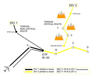
The DATA/Stored Routes function in the MCDU can be used to store up to five possible diversion routes. These routes can be entered into the SEC F-PLN using the SEC INIT prompt. This prompt will only be available if the SEC F-PLN is deleted. *Refer to FCOM/DSC-22\_20-60-40 USING THE SECONDARY FLIGHT PLAN FUNCTION* for further information.
