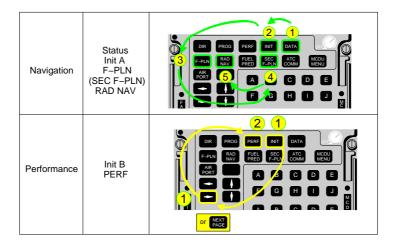
This sequence of entry is the most practical. INIT B should not be filled immediately after INIT A, because the FMGS would begin to compute F-PLN predictions. These computations would slow down the entry procedure.
