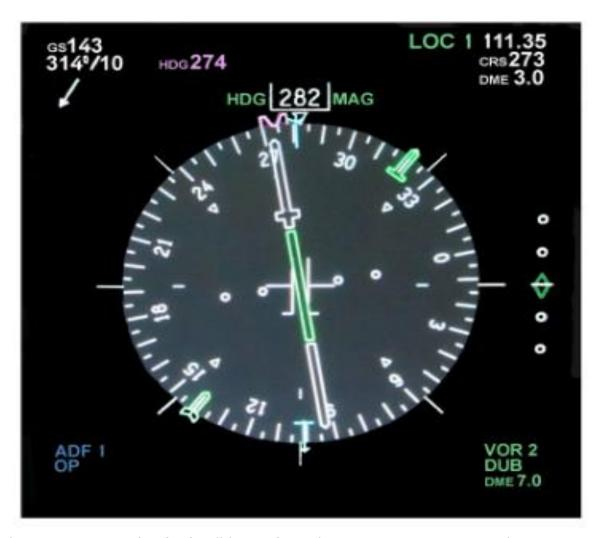
The Navigation Display (ND) will be configured as a VOR compass rose. The instrument has a course selector function. The left (no.1) ND is connected to NAV 1 (left) and the right ND is connected to NAV 2.
