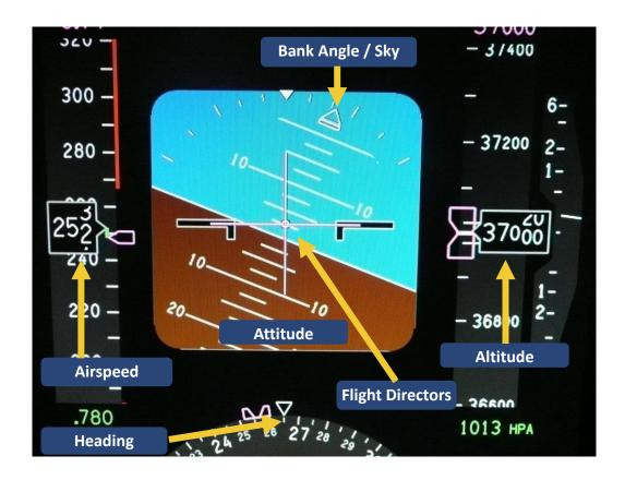
The Primary Flight Displays (PFDs) present a dynamic colour display of all the parameters necessary for flight path control. The displays provide the following information:
